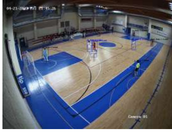
Figure 10: Often the ball (here the blue rectangular) was confused with some reflections of the light on the pitch
